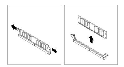
Figure 14. Removing a memory module
